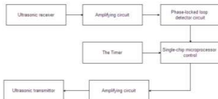
Fig. 2 the principle diagram of ultrasonic ranging system
